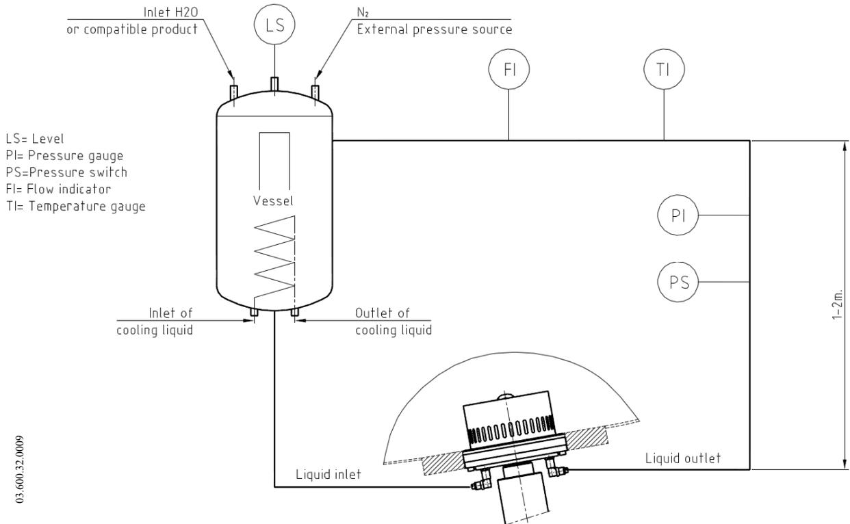
Figure 5.2 Pressure vessel installation scheme
